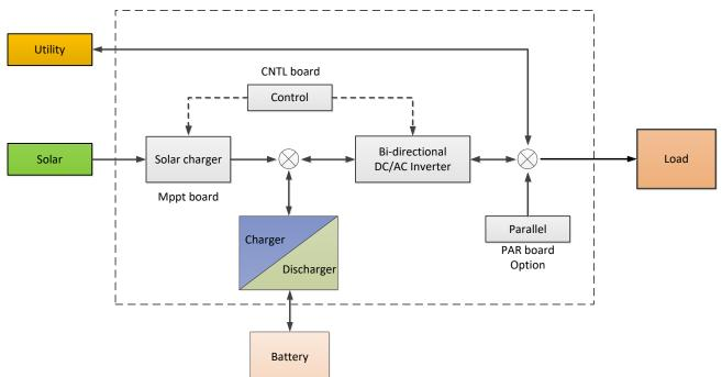
Compare with UPS or normal inverter, INVERTER combines a solar charger inside. Solar charger can be a supplement for battery when there is not grid or for saving energy purpose. And with the solar charger, the inverter can have more working modes than UPS. For detail information please refer to our user manual.
