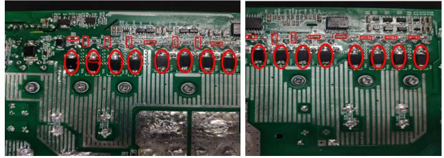
Use multimeter to measure each resistor, find the burnt resistors and replace them; don't need to replace
