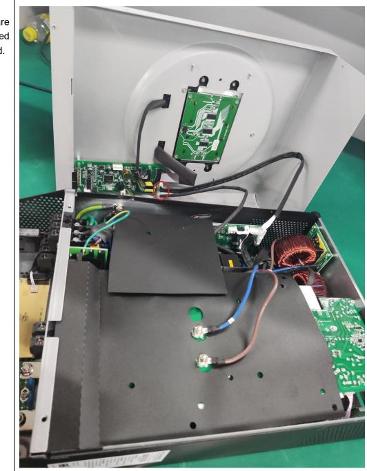
Open the top cover carefully, for there are two cables connected with RGB&LCD board.
